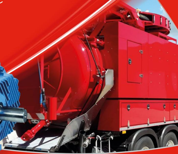
The RB-DV is a range of rotary lobe waste vacuum pumps and blowers applicable for both liquid and dry waste product. Utilising the knowledge from our Robuschi brand of industrial vacuum pumps and blowers, the truck mounted RB-DV provides versatile solutions for transport related requirements. Our portfolio includes six models of varying and extremely high air flow suitable for high volume and 'Super-suction' vacuum waste tankers.
